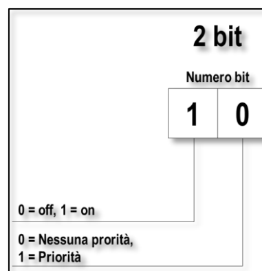
Figure 15 - Forcing command bits
