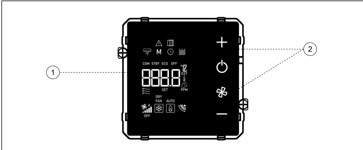
Figure 4a - User interface Easy version: display (1) and backlit touch LEDs (2)
