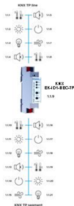
Figure 7 - Segment coupler scheme
